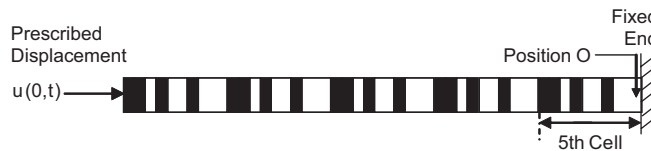
Fig. 12. Banded structure designed for achieving shock isolation over frequency range 0 \leq \Omega^* \leq 50 . The structure is formed from the synthesized unit cell encoded ‘0010110111’, shown in Fig. 2. Its length is L = 5 . The excitation u(0, t) is given by Eqs. (28) and (29). Position O marks a measurement point.
